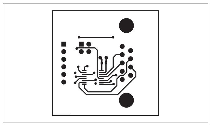
Figure 3. MAX3232PMB1 Peripheral Module PCB Layout—Component Side
