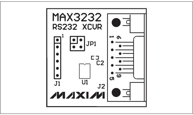
Figure 2. MAX3232PMB1 Peripheral Module Component Placement Guide—Component Side
