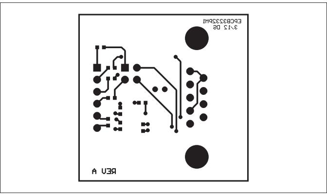
Figure 6. MAX3232PMB1 Peripheral Module PCB Layout—Solder Side
