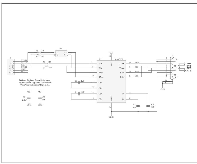
Figure 1. MAX3232PMB1 Peripheral Module Schematic
