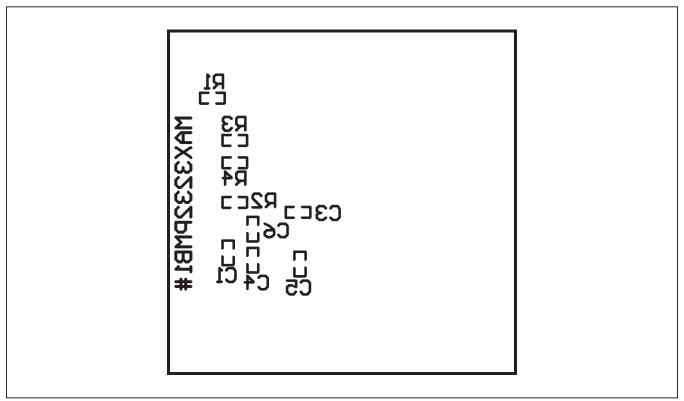
Figure 7. MAX3232PMB1 Peripheral Module Component Placement Guide—Solder Side
