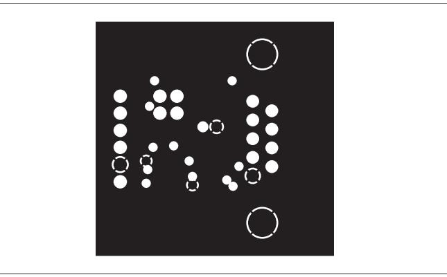
Figure 4. MAX3232PMB1 Peripheral Module PCB Layout—Inner Layer 1 (Power)
